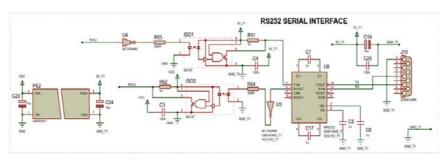
Fig. 5 Galvanically isolated RS232 port
