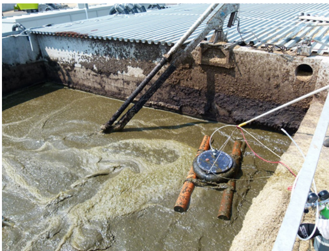
Fig. 3 Picture of the positioning of the flux chamber for sampling in the mixing tank
