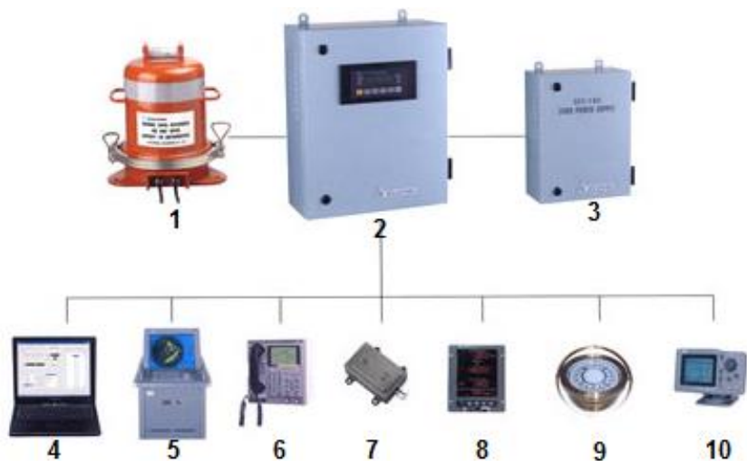
Fig. 1 Componentele unui sistem VDR (Voyage Data Recorder) [3]
