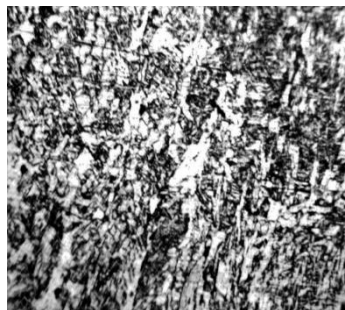
Fig. 11 Proba E1T, SUD, atac Nital 2%, 100X
