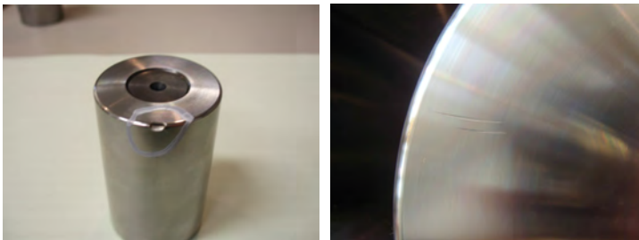
Fig. 6 Role cu defect de material
