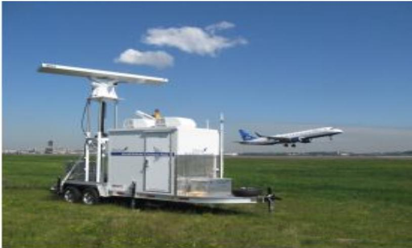
Fig. 6 Detects MERLIN Aircraft Birdstrike Avoidance
