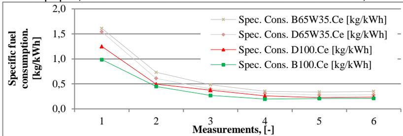
Fig. 3 Experimental test results concerning specific fuel consumption
