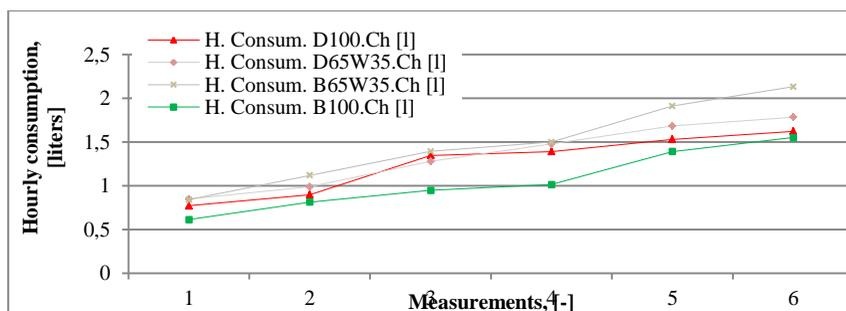
Fig. 2 Experimental test results concerning hourly fuel consumption
