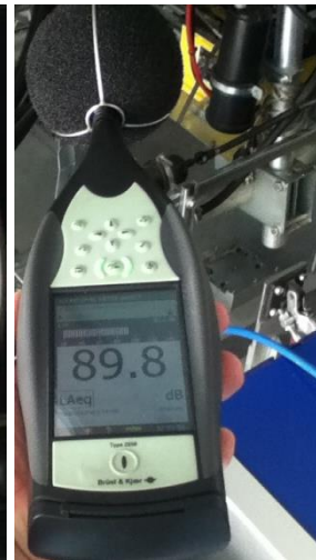
Fig. 9 Determining noise actual value at approximately 3500 rpm
