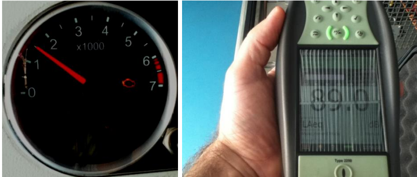
Fig. 6 Determining the sound level at 1500 rpm
