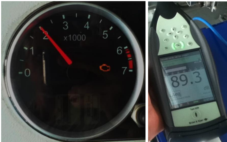
Fig. 7 Determination of sound level at 2000 rpm on Ford S.I. engine
