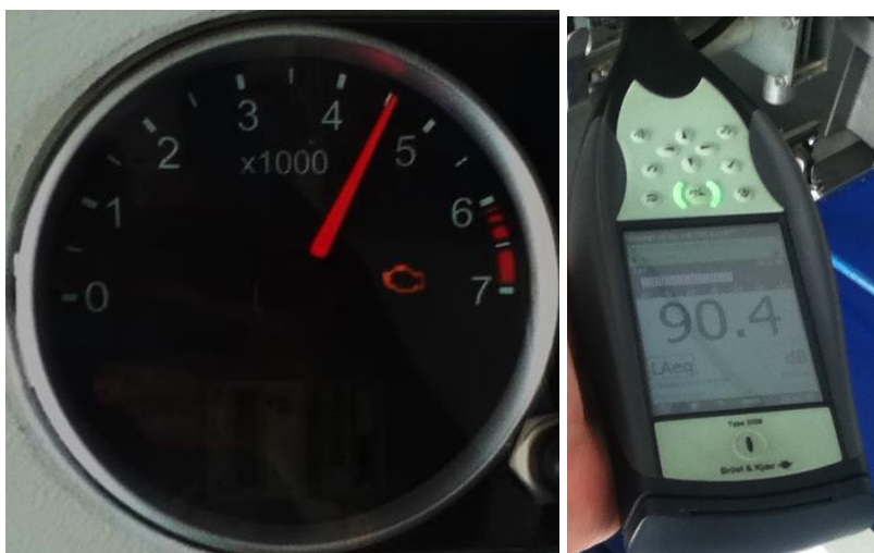
Fig. 11 Show of basic measurement values concerning noise emissions at 4500 rpm
