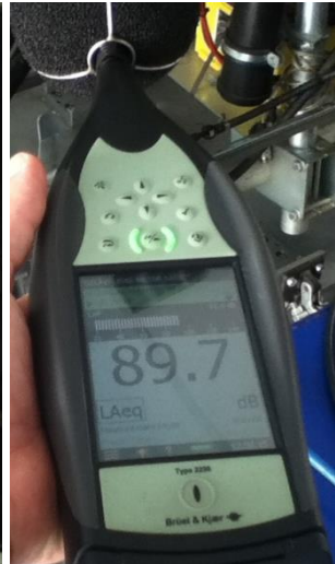
Fig. 8 Measurement of noise level at 3000 rpm of engine's crank shaft
