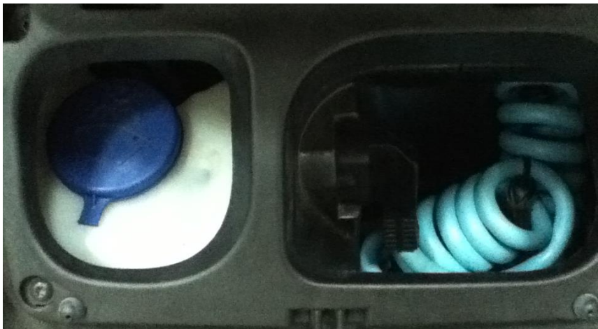
Fig. 7 Supplies cover in front of Renault Twizy, for liquid and electric energy
