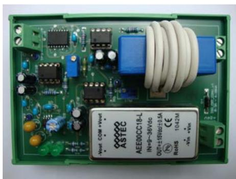
Fig. 3 The current adapting block (0.5V AC - 4..20mA)
