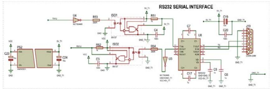
Fig. 5 Galvanically isolated RS232 port
