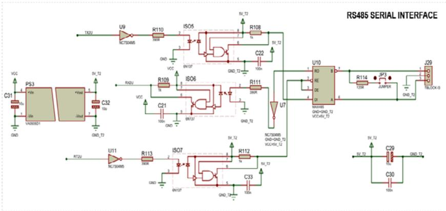
Fig. 6 Galvanically isolated RS485 port
