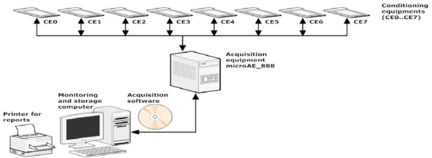
Fig. 1 Structure of the acquisition system
