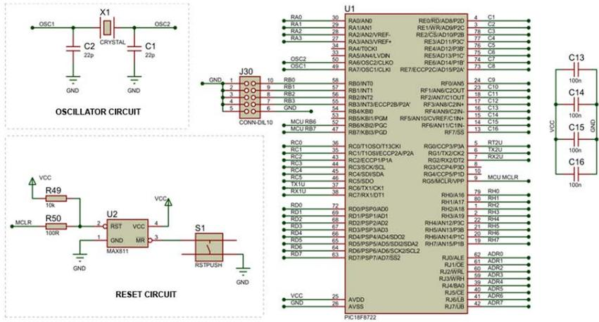
Fig. 4 The connection of RESET circuit and external oscillator to the microcontroller
