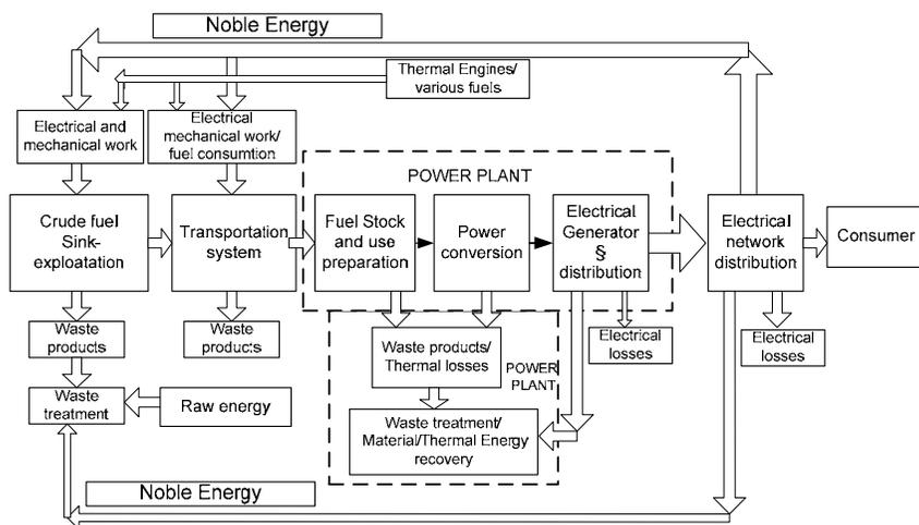
Fig. 2 Electrical energy production/consumption diagram applied to a thermal power plant
