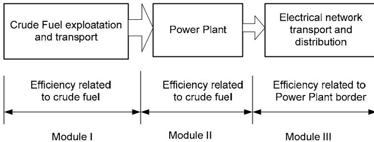
Fig. 3 The efficiencies diagram for the electrical energy chain produced by a power plant
